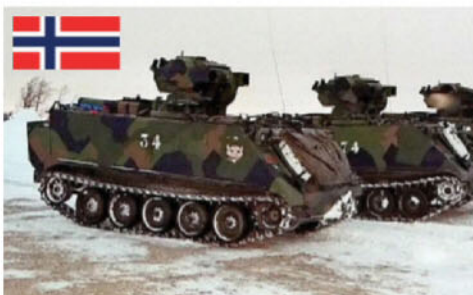
Taking its lead from the US M-113, the Norwegian Model-142 uses a TOW2 guided missile system to blast tanks out of the battlefield
